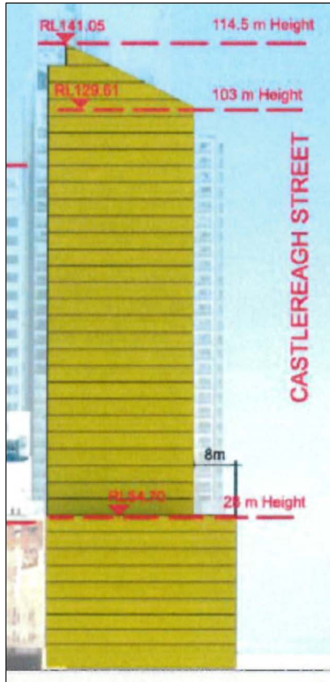
Figure 8: The approved Stage 1 building envelope, illustrating the approved roof form and slope
