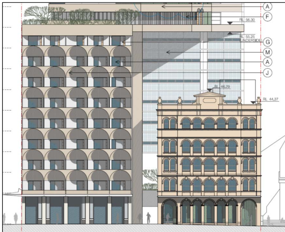
Figure 18: The detailed design of the podium and Porter House (lodged as Stage 2 DA), illustrating the separation between buildings at 3.8 metres
